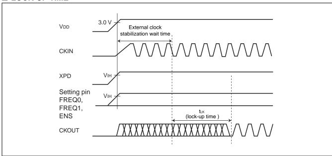
If the XPD pin is fixed at the "H" level, the maximum time after the power is turned on until the set clock signal is output from CKOUT pin is (the stabilization wait time of input clock to CKIN pin) + (the lock-up time "tuk"). For the input clock stabilization time, check the characteristics of the resonator or oscillator used.
