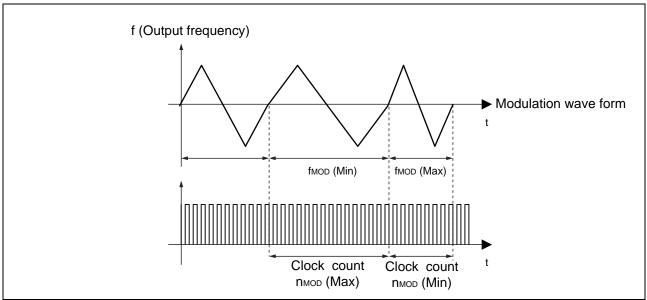
MB88153A contains the modulation period to realize the efficient EMI reduction.
