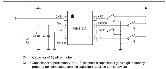
: Impedance matching resistor for a circuit on a board
