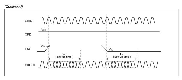
When ENS pin is controlled for enable modulation, it is necessary for the stably clock output from CKOUT pin to wait lock-up time (tlk).
